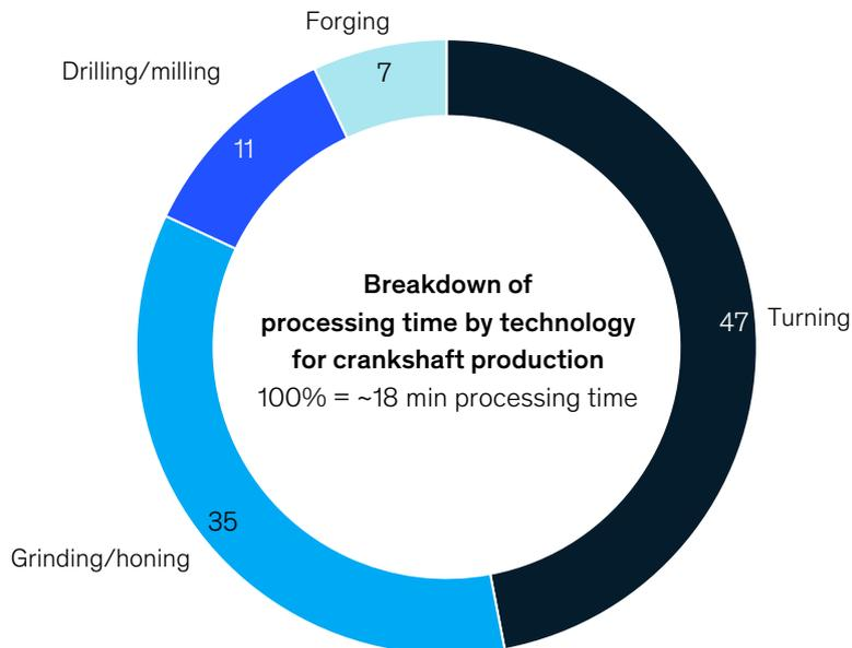
Due to developments in global new-car sales, crankshaft demand for 2020 was projected at 86 million crankshafts. Because of the increasing number and share of cars with electric powertrains, only 62 million crankshafts are expected to be required in 2030. Crankshaft production had a capex of USD 76 million in 2020; compare this to an expected capex of USD 25 million in 2030, based on the powertrain shift and assumed reuse rates.
